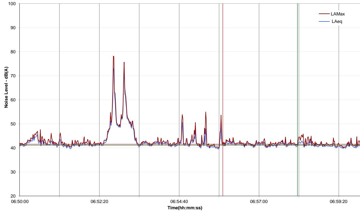
Note: Gaps in graph are periods where SLM was paused to exclude extraneous noise from measurements.
