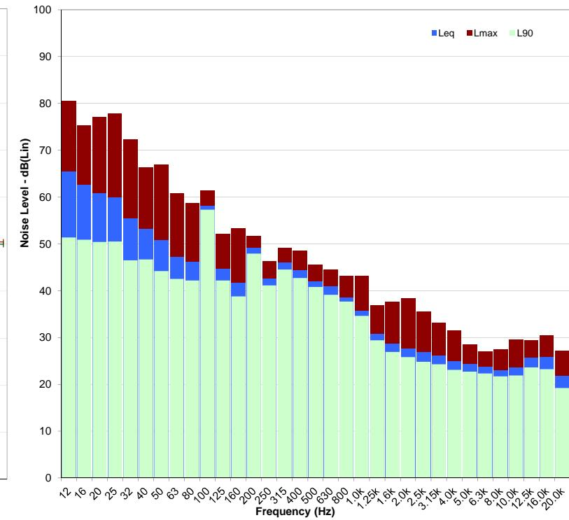
Note: Gaps in graph are periods where SLM was paused to exclude extraneous noise from measurements.
