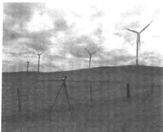
Figure 3. Monitoring wind turbine noise at an operating wind farm, Waterloo, South Australia. Notice that the blades of the four turbines have closely matched phase. Considered as a random event, the chance of 4 turbines having all phases equal to within 5^\circ of each other are (5/360)^3 \approx about 1 in 2 million. Photo. EPA South Australia, with permission.
