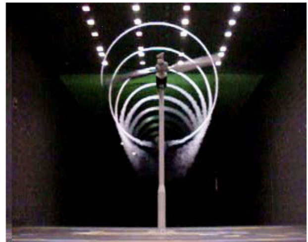
Fig. 3. NREL Phase IV experiment with smoke trail (Hand, 2001).
